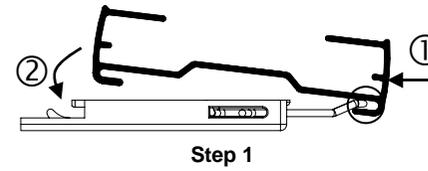
Insert the Bracket Clip into the screw from the notch.
