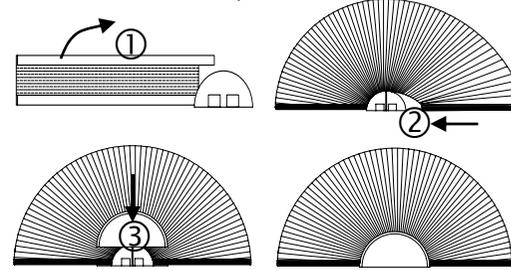
For Quarter Round, Arch on Top, Angle Top, and Half Eyebrow (take Quarter Round as example): Open the shade and place the rail into the bottom of 90°center support tightly, and then install the front and back 90°center templates:
