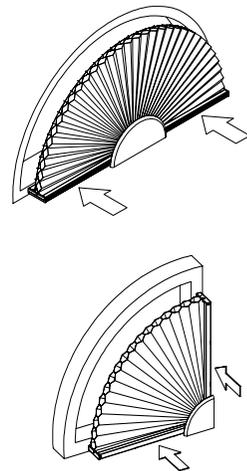
Place the front groove of the rail into the front iron wire of the bracket and then push forward to make the back groove of the rail snap into the back groove of the bracket.
